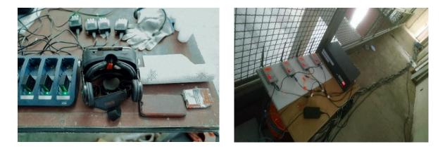
Figure 10. Hardware components: VR glasses and batteries (on the left), and switch and receivers (on the right).
