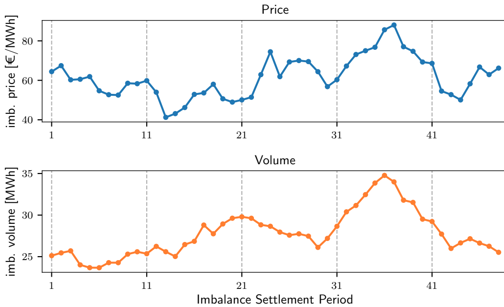
Figure 2.29: Standard deviation of imbalance prices (top) and volumes (bottom) for each Imbalance Settlement Period.
