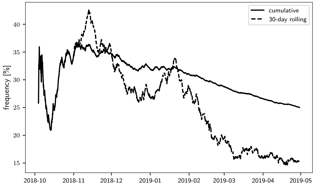
Figure 2.45: Cumulative (solid line) and 30-day rolling (dashed line) frequency of imbalance prices anomalies.
