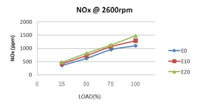
Fig. 5. High-speed NO<sub>x</sub> emissions from engines under different fuel mixing ratios
