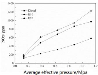
**Fig. 6.** Effect of ethanol addition ratio on NO<sub>x</sub> emissions
