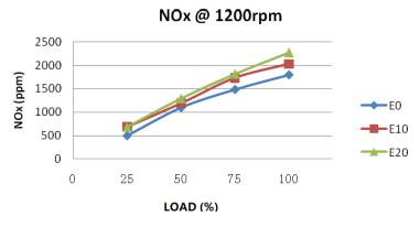
Fig. 3. Low engine NO<sub>x</sub> emissions under different fuel mixing ratios
