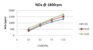
Fig. 4. Medium-speed NO<sub>x</sub> emissions from engines at different fuel mixing ratios
