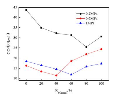
Fig. 7. CO emissions vary with Rethanol under each load
