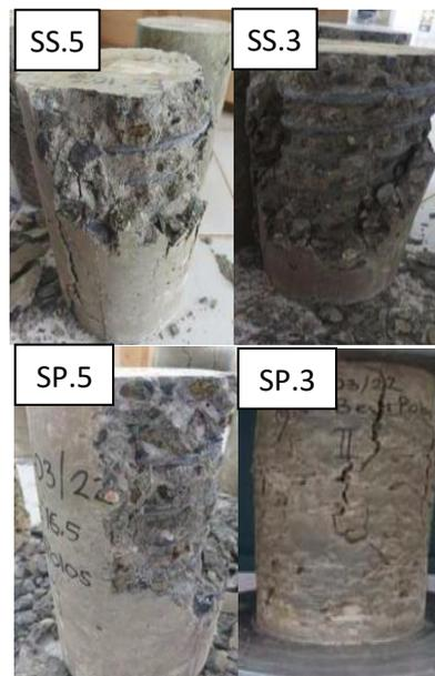
Gambar 8. Pola retak sengkang
