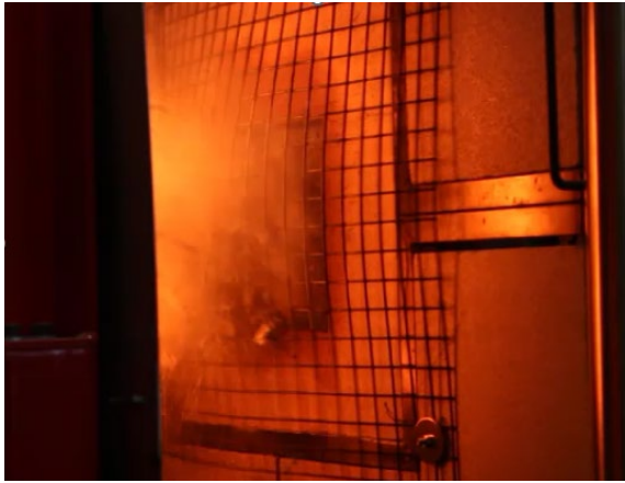
Figure 12 Still frame of specimen Ref-CFRP-A with debris flying towards the RPA
