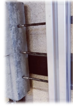
Figure 10 LPs measuring elongation.
