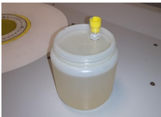
Figure 4-3 – Experimental phantom with lesion designed by Khalesi et al. [7]
