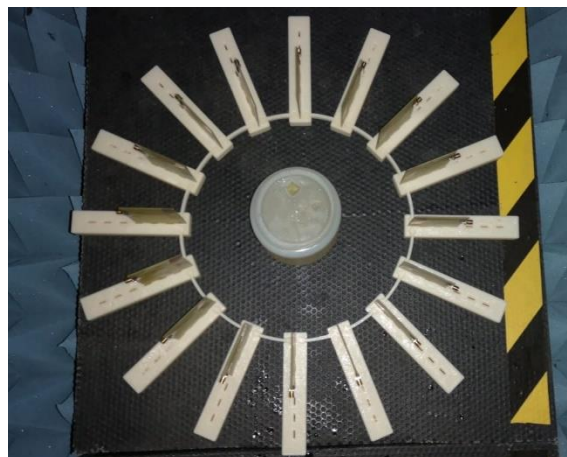
Figure 4-9 – Measurement test B – Healthy phantom present
