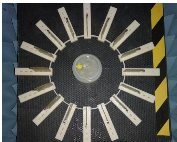
Figure 4-10 – Measurement test C – Phantom with lesion at Pos1
