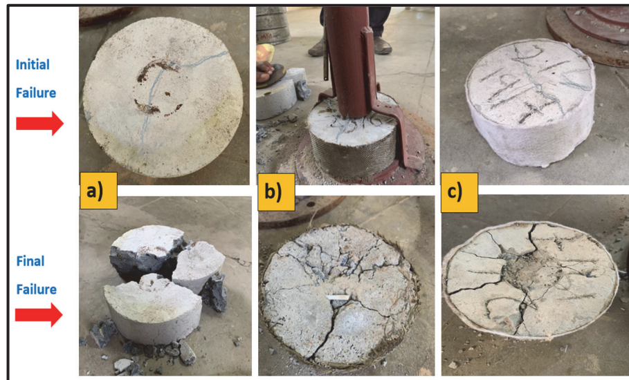
Figure 11: Crack formation during initial and final failure (a) Plain concrete sample (b) Basalt fiber wrapped sample and (c) Geotextile fiber wrapped sample.
