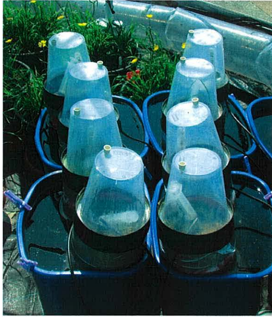
Figure 5.1: Mesocosms with the headspaces on. The neoprene seal is between the transparent pot and the plastic mesocosm liner. Gas samples are taken through the rubber septa at the top of the headspace chamber.
