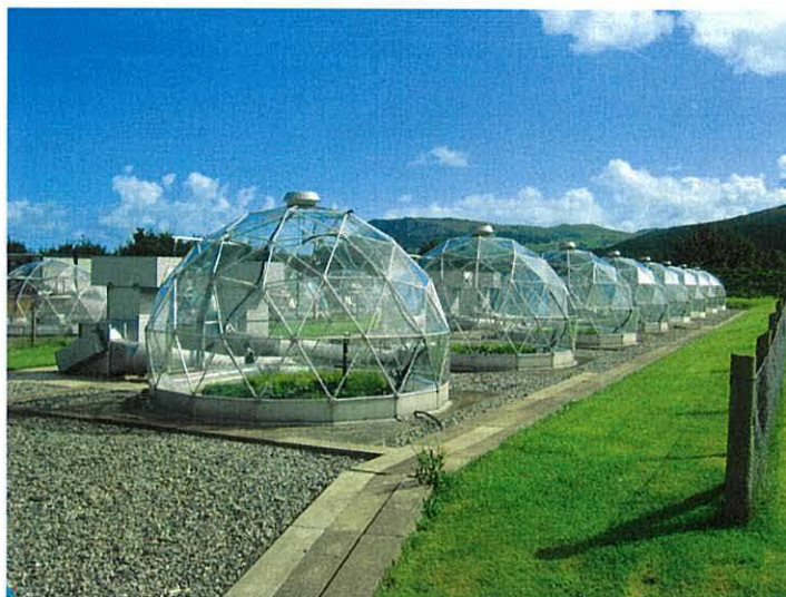
Figure 2.2: Solardomes at Abergwyngregyn, situated on an East-West line to minimise differences in shading.
