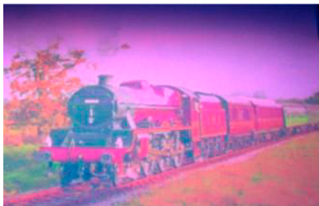
FIGURE 15 Colour image ink-jet printed on non-fluorescently brightened paper using luminophores inks, viewed under 254 nm UV illumination.
