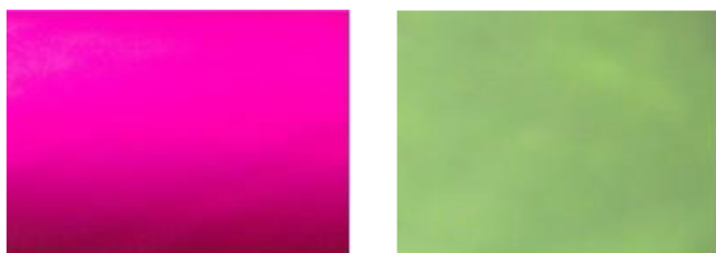
FIGURE 12 Polyester fabrics “dye” with the red and green disperse luminophores, using a high-temperature “dyeing” process, viewed under 254 nm UV radiation.
