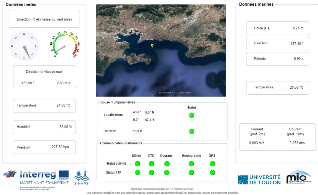
Fig. 16: Real-time visualisation of data obtained from the monitoring system (ixbuoy-toulon website, 2022)
