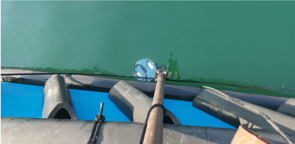
Fig. 32: V-ADCP mounted on side of the vessel during monitoring campaigns
