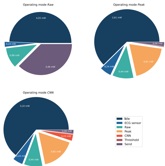
FIGURE 20. Estimation of energy consumption for each task of each operating modes at 60 bpm.
