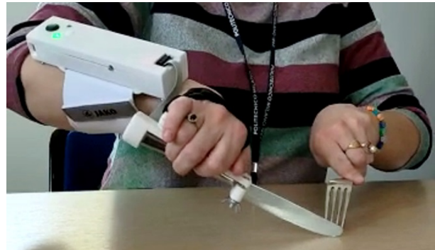
Fig. 4: Demo of e-KIRO used in cutlery handling. The control board unit is attached to the user’s forearm.
