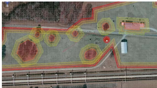
Fig. 4.2 Geofencing example, the stay-in region is the land parcel, while several stay-out regions are defined to avoid obstacles [34]
