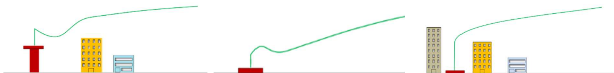
Fig. 6.2 From left to right, Elevated conventional, conventional and vertical takeoff profiles [50]
