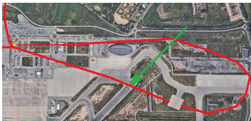
Fig. C.4 eVTOL procedures crossing LEBL runway 20 threshold (green arrow) [own source, Google Earth]
