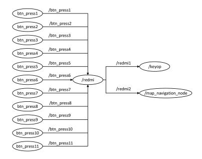
Figure 3. Android device communication with the robot control nodes.
