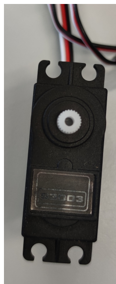
Figure 8: One of the replacement Futaba S3003 servo-motors.
