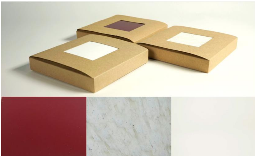
Figure 3. Material samples. In order from left to right: M1, raw material called Altuglas; M2, recycled material from Carpintería Plástica; and M3, recycled material called Syntal.
