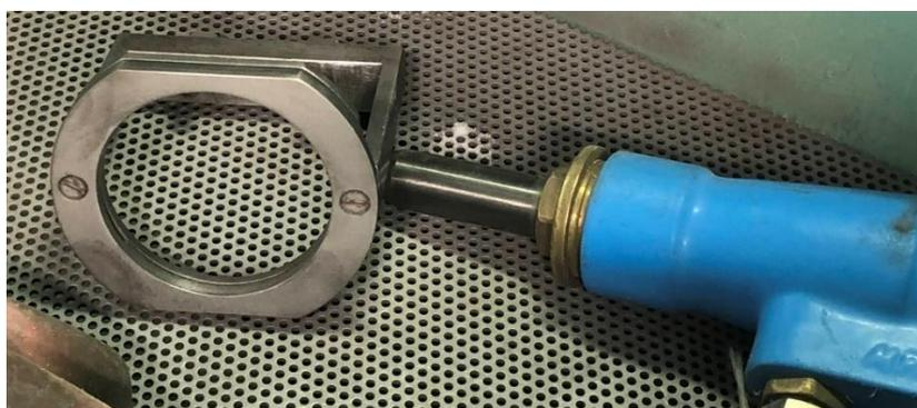
**Figura 7.7.** Base celda interior sometida a chorro de arena.
