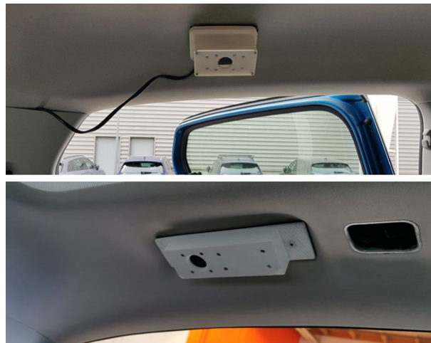
Fig. 7 Camera module installations in the SEAT concept car (top) and Aalto research vehicle (bottom)
