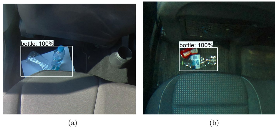
Fig. 27 Two instances of the bounding box merging for items placed in close proximity to each other. The image in a depicts items from the same trained class and the image in b depicts items from two different trained classes
