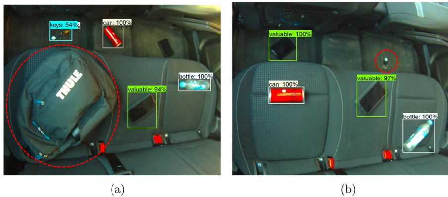
Fig. 28 Two examples of predicted images with a high quantity of items scattered across the seating area. Red dotted circles correspond to instances of undetected items ( a bag and b keys)
