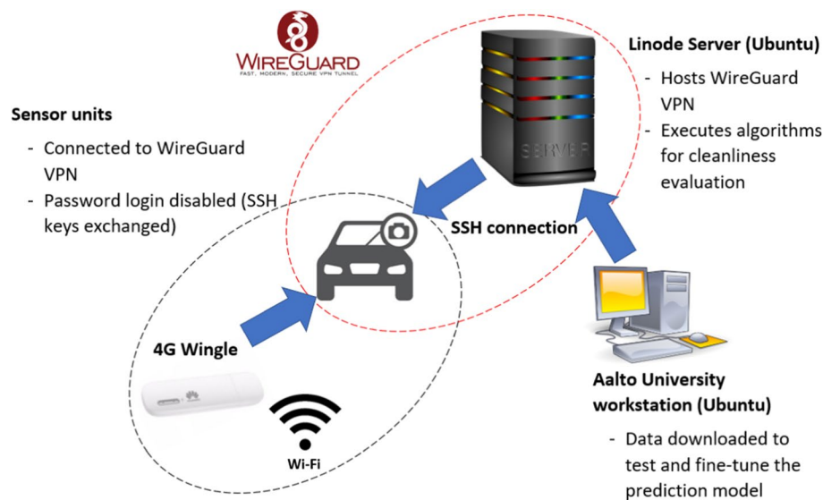
Fig. 12 Communication setup of the detection system
