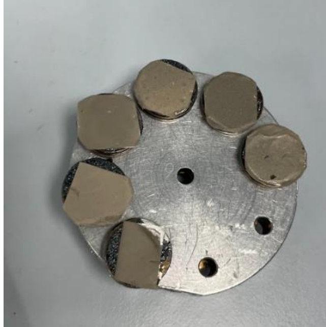
Figure 11. Samples treated prior entering SEM microscopy. It can be appreciated the thin layer above consisting in carbon particles
