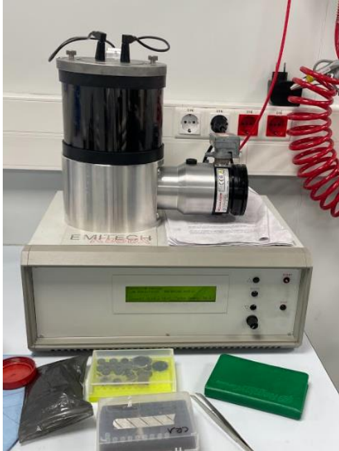
Figure 12. Automatic carbon coater used for preparing the samples before entering to the SEM microscopy.
