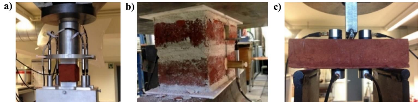
156 157 Figure 1 Experimental setup for small samples: a) compression test on cubes, b) compression test on 158 couplets and c) three-point bending test on small beams (clay brick shown here). Colour figure available in 159 online version.
