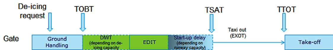
Figure C.1: Gate de-icing process in AMS[10]
