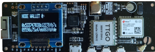
Figure 2. LoRa device: T-Beam board with LoRa radio.
