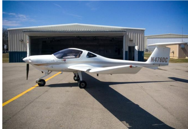
Fig.3.5. Tadpole Fuselage. Diamond DA20 C-1
