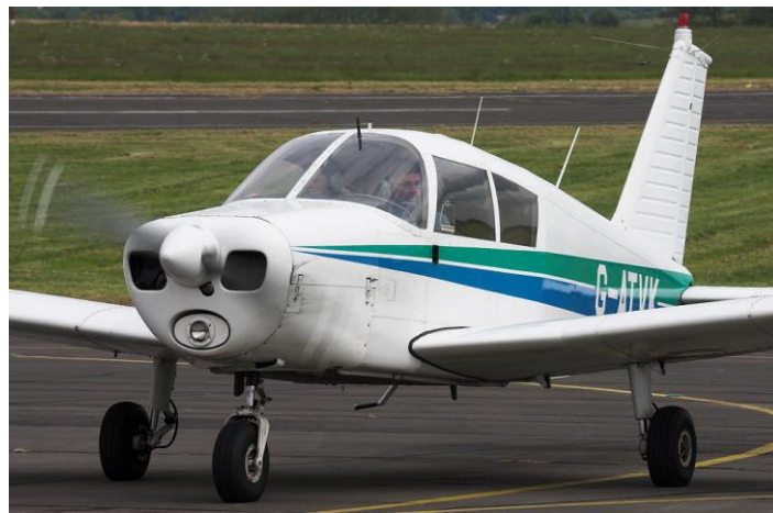
Fig.3.3. Frustum Style Fuselage. Piper PA-28 Cherokee [31]
