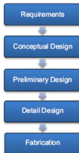
Fig.1.2 Elementary outline of an aircraft design process [12]
