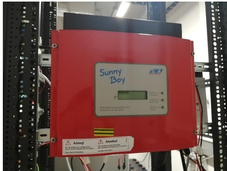
Figure 3.2. An image of the SB700 used in the simulations for the project.
