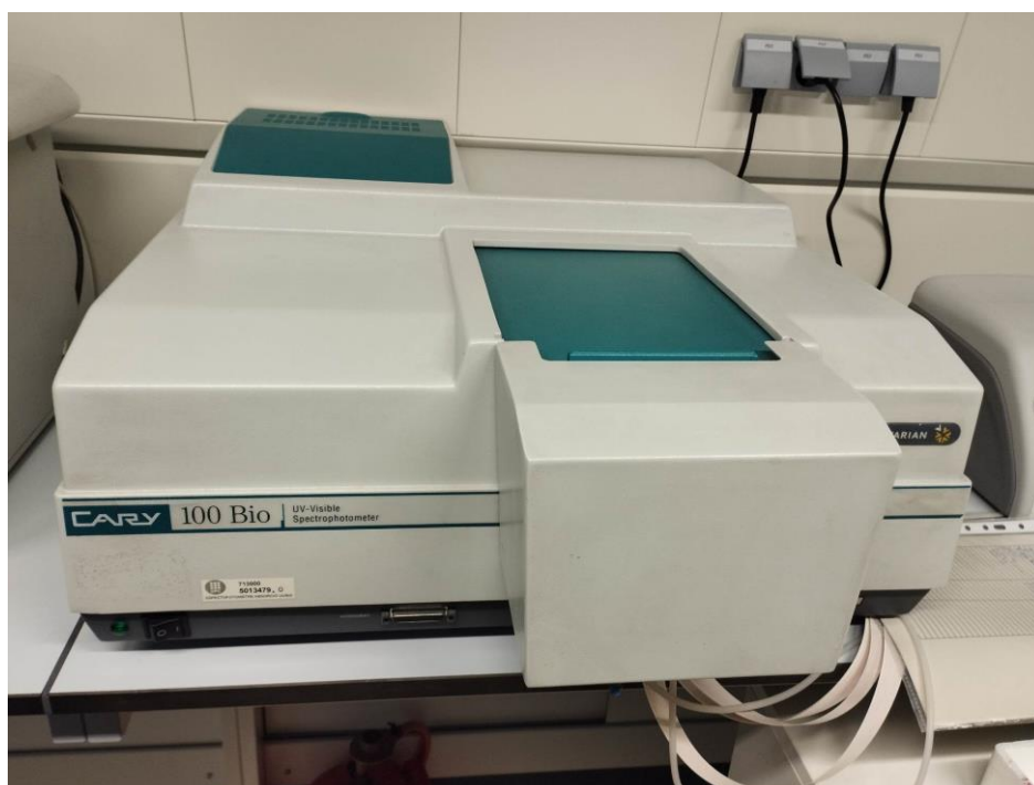
Fig. 2.5.2. The UV-Vis Cary 100 Bio spectrophotometer used in the study.
