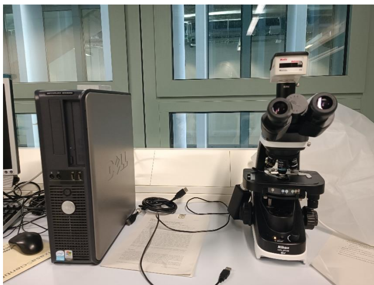
Fig. 2.3.1. The Nikon Eclipse Ei optical microscope used for the fiber optimization.
