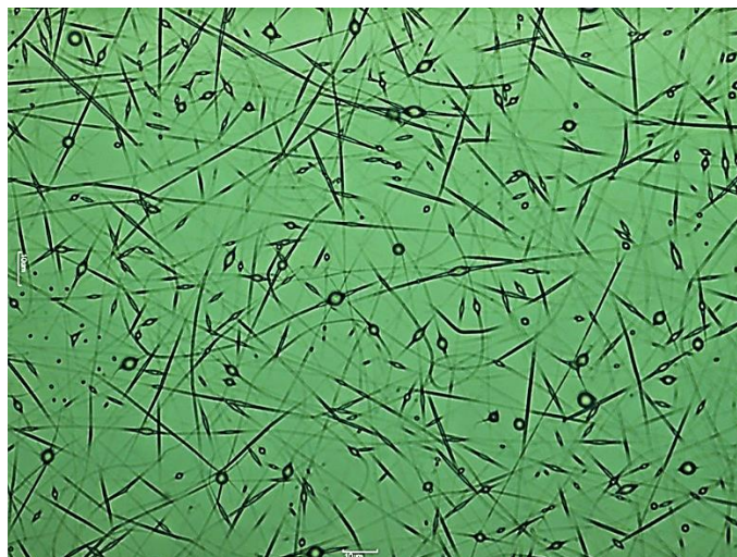
Fig. 3.2.1.7. PLA/ HPMC electrospun solution after 5 days of its preparation
