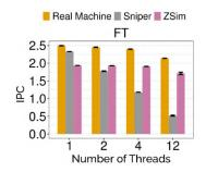
Fig. 2: IPCs with prefetcher disabled on ZSim and Sniper simulations and on the real execution.
