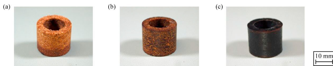
Fig. 6. Appearance of compacts obtained at a binder content, BC , of 40 wt% and a temperature, T , of (a) 180, (b) 190, and (c) 200 °C.
