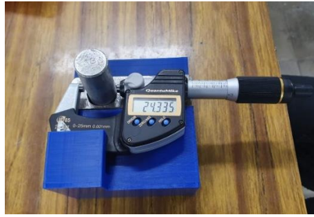
Fig. 1. Example of a 3D printed support used to measure the shaft diameters
