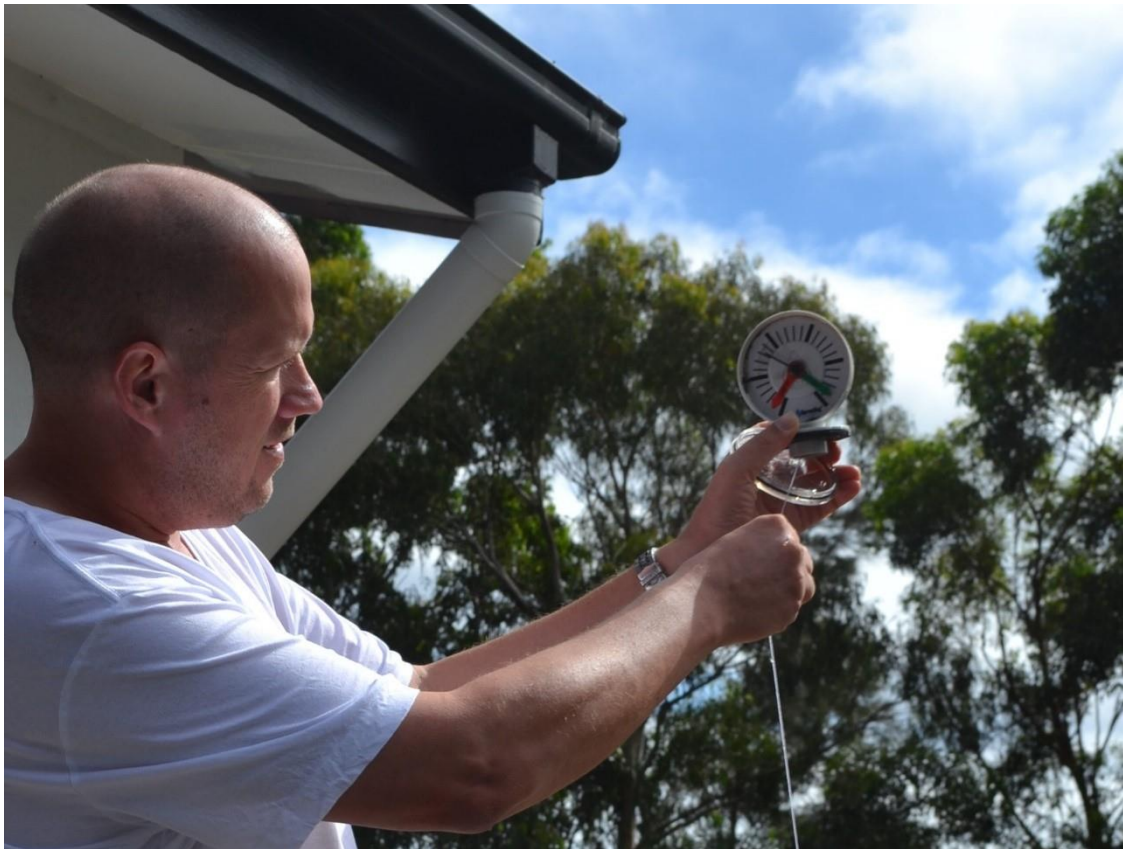
Figure 5.4: Dave demonstrating the new ‘floaty’ gauge he’s installing on a rainwater tank.
