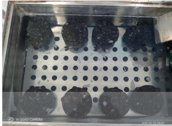
Figure 3.20 Samples in water bath at 25°C
