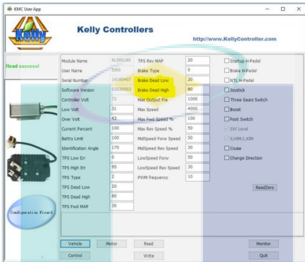
Figure 3:8 Graphical user interface of Kelly Controller User Configuration software.
