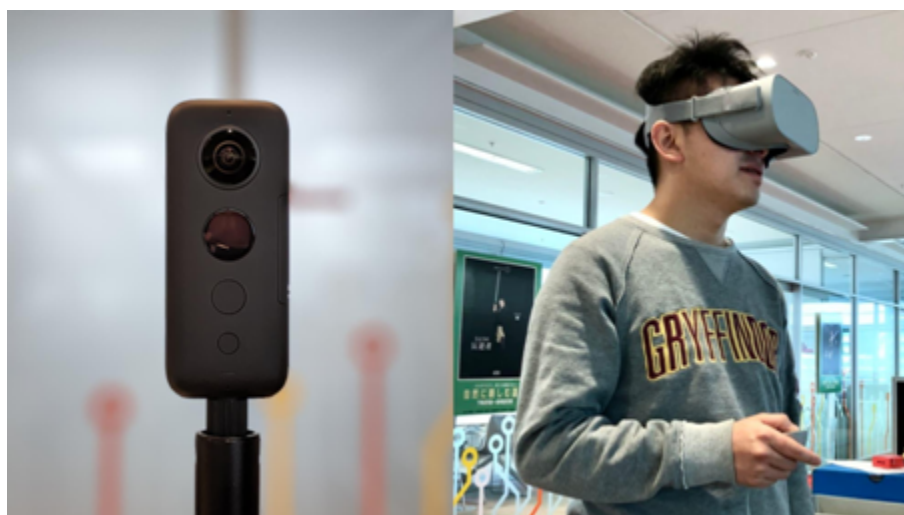
FIGURE 2.1: One of the 360-degree cameras available on the market (left); a viewer watching a 360-degree video (right).
