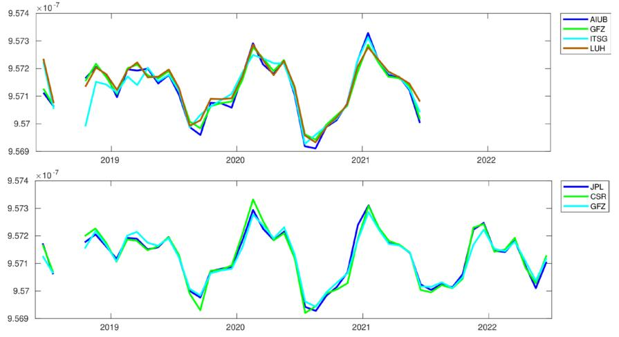
The accelerometer transplant product has a major impact on gravity field coefficient C<sub>30</sub> (artefacts with 320d-period).
