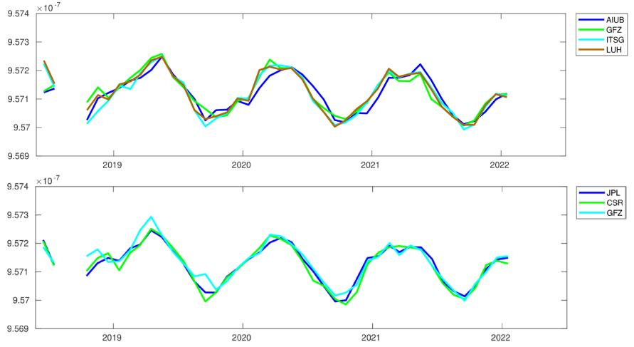
The accelerometer transplant product has a major impact on gravity field coefficient  $C_{30}$ . The artefacts in  $C_{30}$  are remarkably reduced with the G3P/new JPL-ACT.
