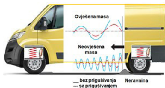
Slika 2 Niskofrekventne i visokofrekventne vibracije vozila Figure 2 Low-frequency and high-frequency vehicle vibrations
