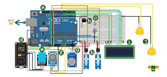
Figure 3. Design of the IdeAir device.
