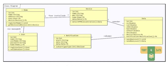
Figure 5. IdeAir refined class diagram.
