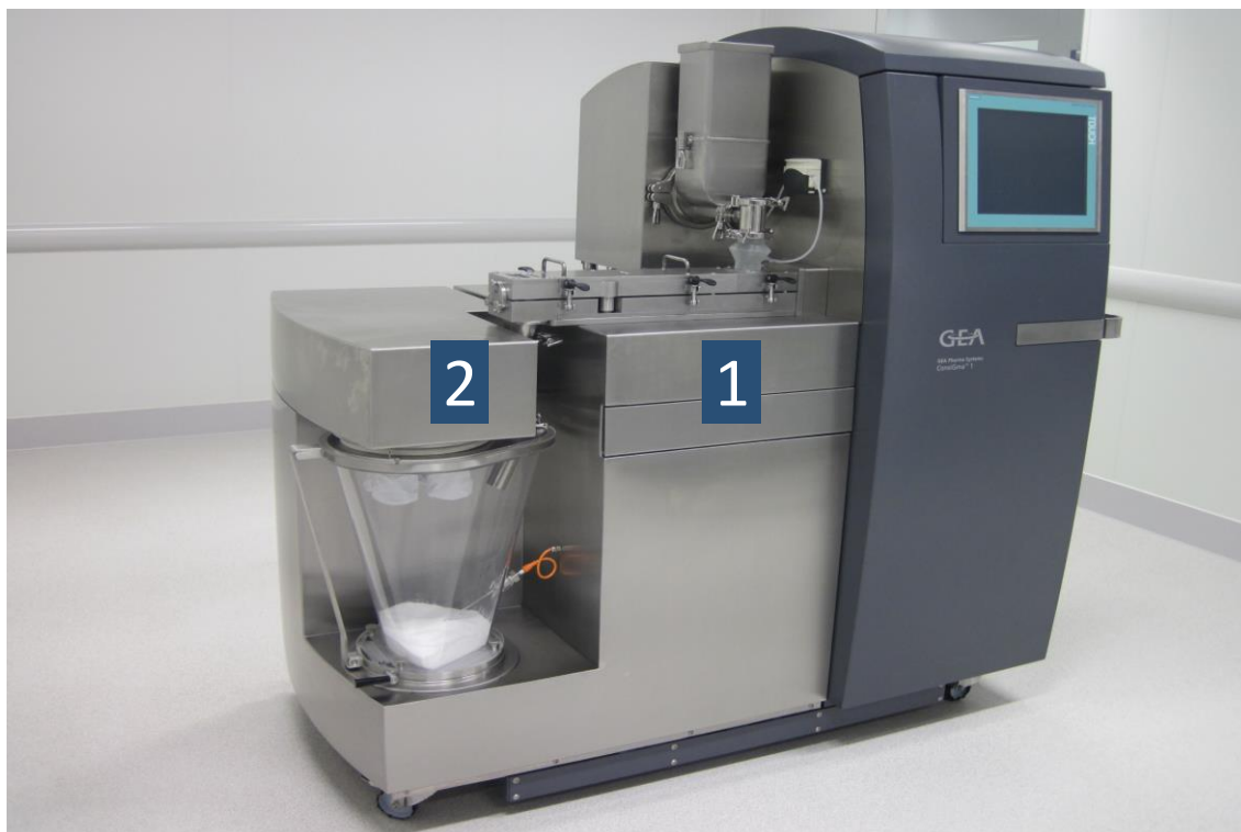
Figure 1: ConsiGma™-1 mobile laboratory unit: 1. Twin screw granulation module, 2. Fluid bed dryer module (1 segment).
