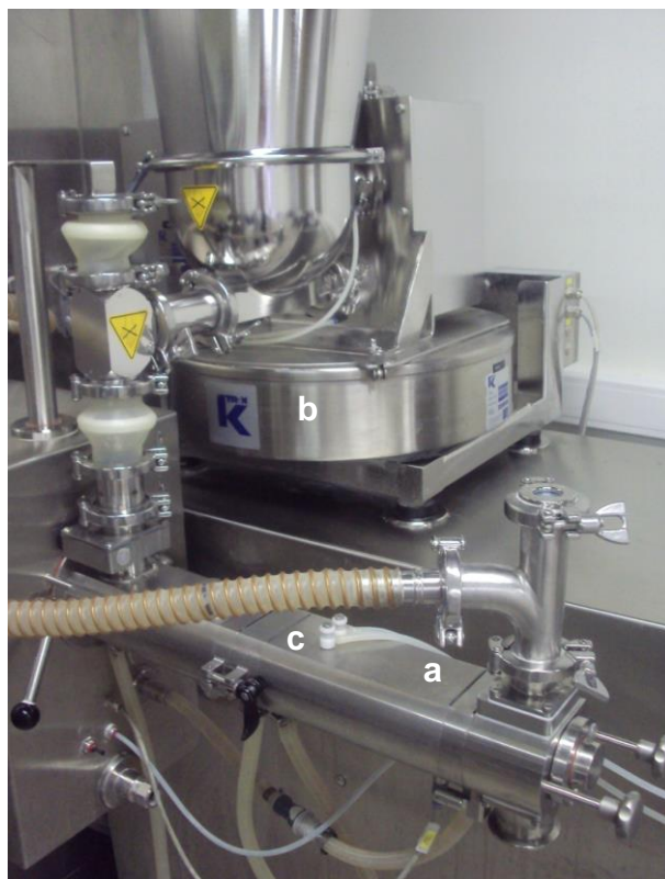
Figure 1: Consigma TM -25 granulation unit: high-shear twin screw granulator (a) with K-Tron KT20 loss-in-weight feeder (b) and gravimetric liquid addition on both screws (c).
