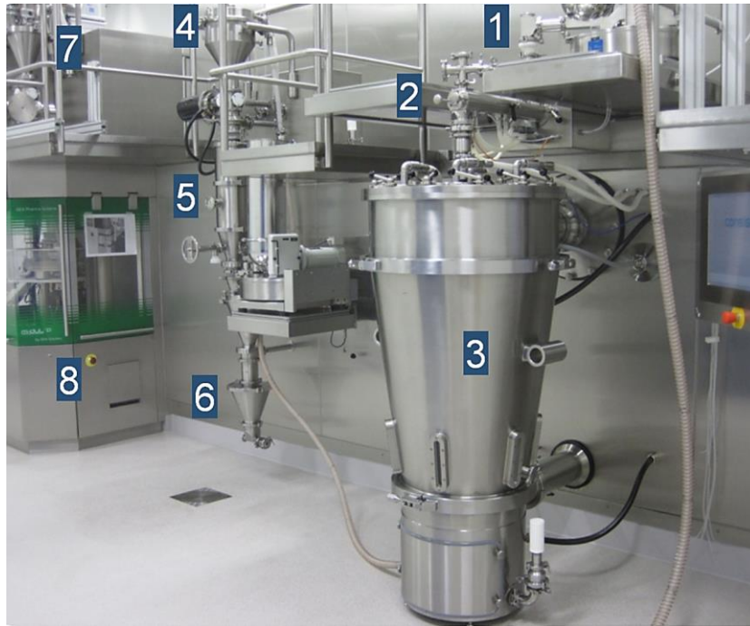
Figure 1: Consigma™-25 continuous tablet manufacturing line: 1. Powder dispensing, 2. Screw-based wet granulation module, 3. Segmented fluid bed dryer, 4. Granule conditioning unit with 5. Quadro® comil® and 6. Blender (external phase), 7. Blender (lubricant), 8. Modul™ P tablet press.
