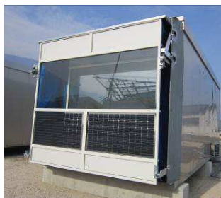
BiPV facade on PASSYS cells.
