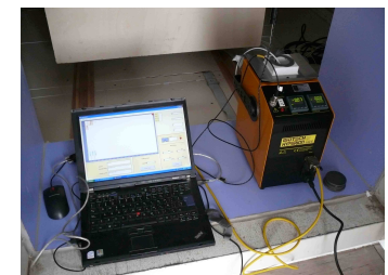
Calibrating temperature sensors in a controlled bath in the LCCE premises.
