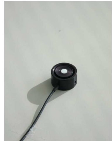
Photometer head for determining luminance (upper image) and lighting levels (lower image)
