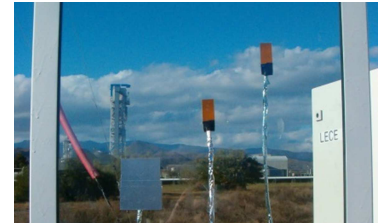
Pt100 used for surface temperature measurements
