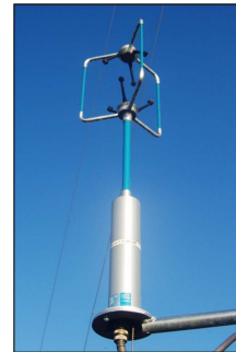
3D ultrasonic anemometer
