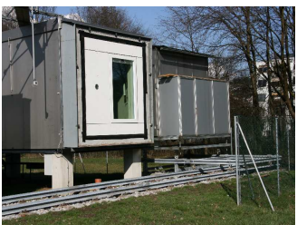
Test cell and Cold-Box in parking position
