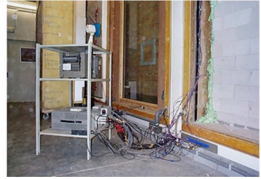
Data logging of the building elements: all sensors are connected to the logger via plug-in-cards.
