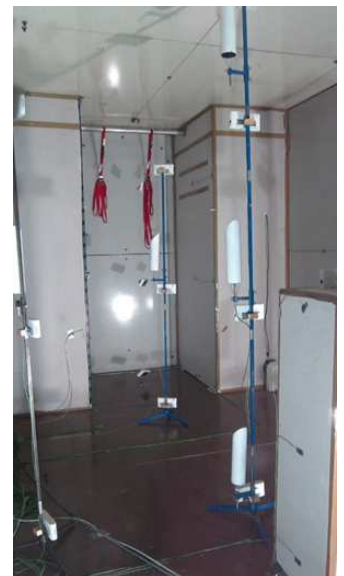
Interior of test cell for measurement of the air exchange efficiency
