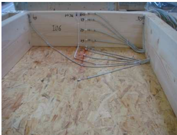
Sensor positioning in a wall assembly
