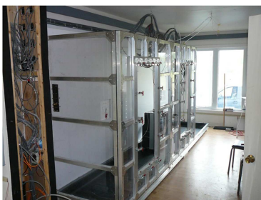
Enclosure for control of interior Temperature, RH, and pressure.
