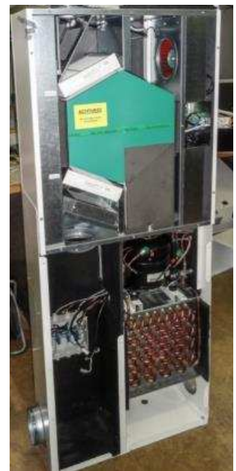
MVHR-unit with micro-heat pump (Project iNSPiRe)
