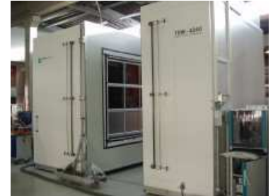
Test of building components in hot box.
