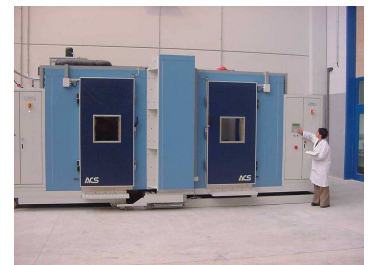
Guarded hot box for opaque walls (according to EN ISO 8990)
