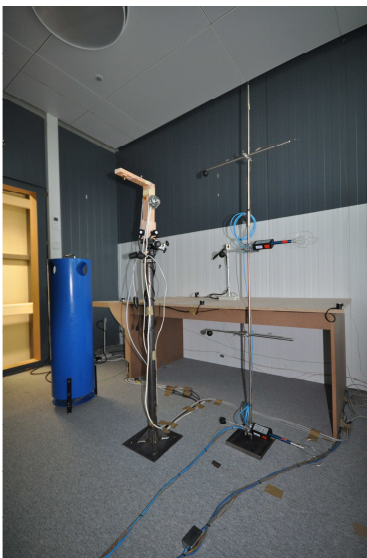
Sensors for air temperature, radiation and air speed are set up in the middle of the test room.
