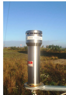
2D ultrasonic anemometer
