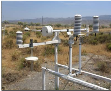
Different devices measuring outdoor air temperature, using natural and forced ventilation
