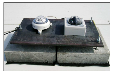
Photo of pyranometers on the roof of the Cube, Wilhelm Lambrecht pyranometer at the left and BF3 at the right
