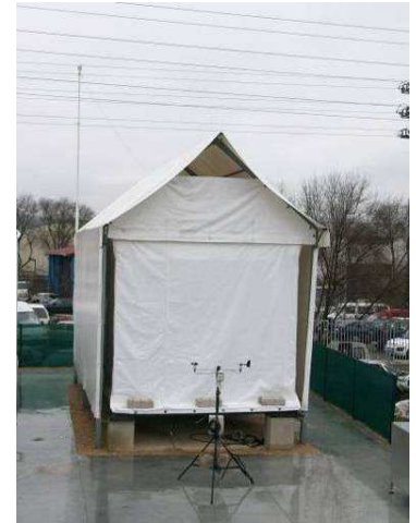
EGUZKI without sample and protected with a tarpaulin. Meteorological station is located 10 m high. Air temperature, velocity and direction in front of the sample.
