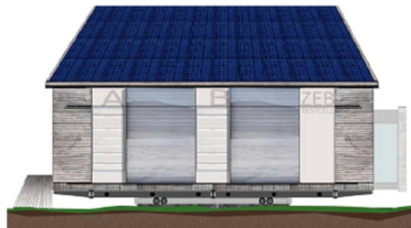
South façade, showing the two interchangeable façade elements of the calorimetric cells.
