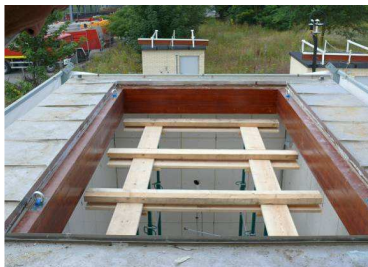
ILARGI: Frame for roof samples.
