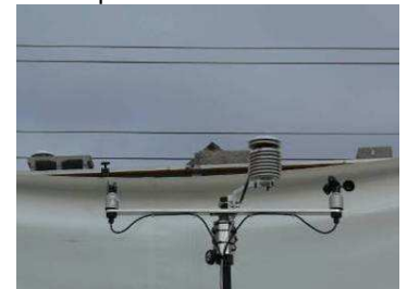
ILARGI air temperature, velocity and direction in the height of the roof.
