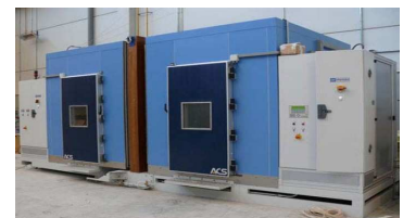
Guarded hot box for windows (according to EN ISO 12567)
