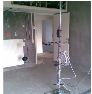
Air, globe and surface temperature sensors, humidity sensors, lux sensor and heat flux sensor in one side-by-side room in EnergyFlexLab.
