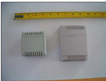
Installed indoor air temperature (left) and relative humidity sensors (right)
