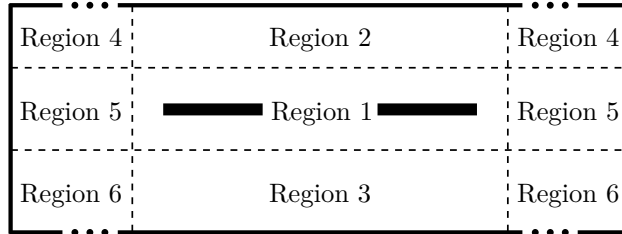
Figure 3.12: Subgridding regions to discretize the differential stripline pair
