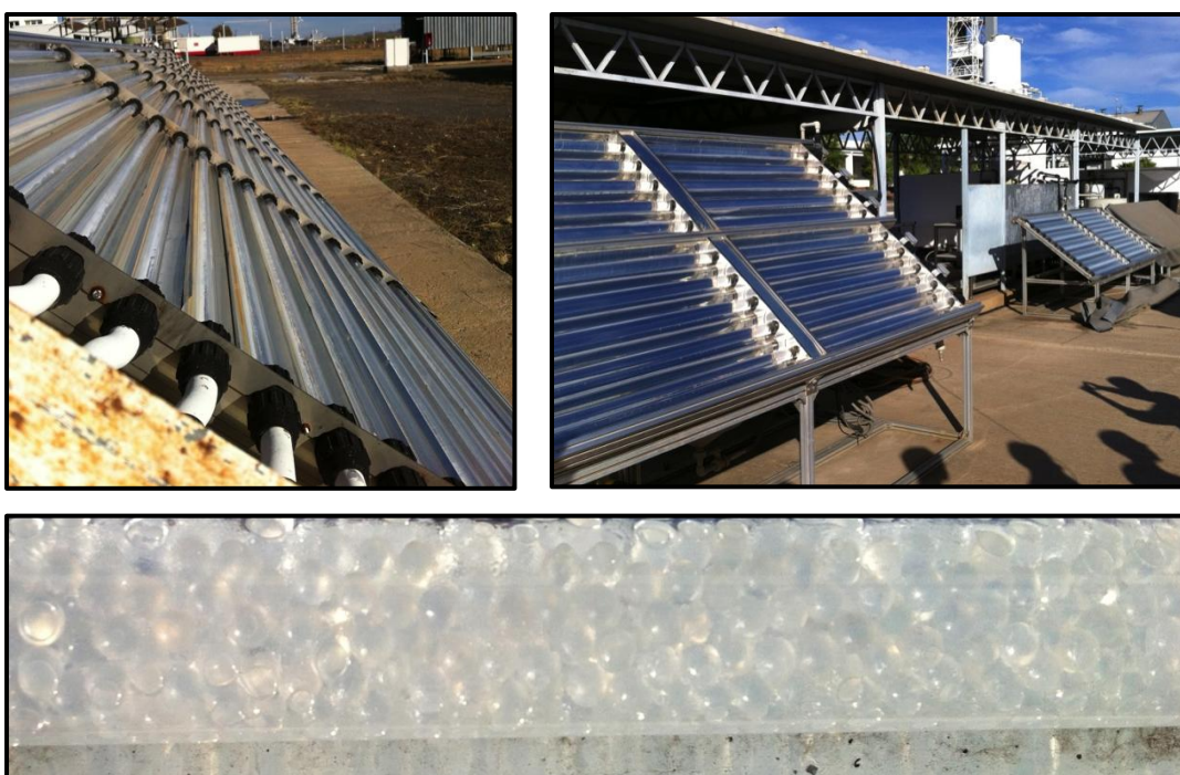
Fig. 6.2 (Top) Solar photocatalytic reactors at Plataforma Solar de Almeria, Spain, (Bottom) \text{TiO}_2 coated glass spheres with \text{Ø} 5 mm (pictures taken by author).
