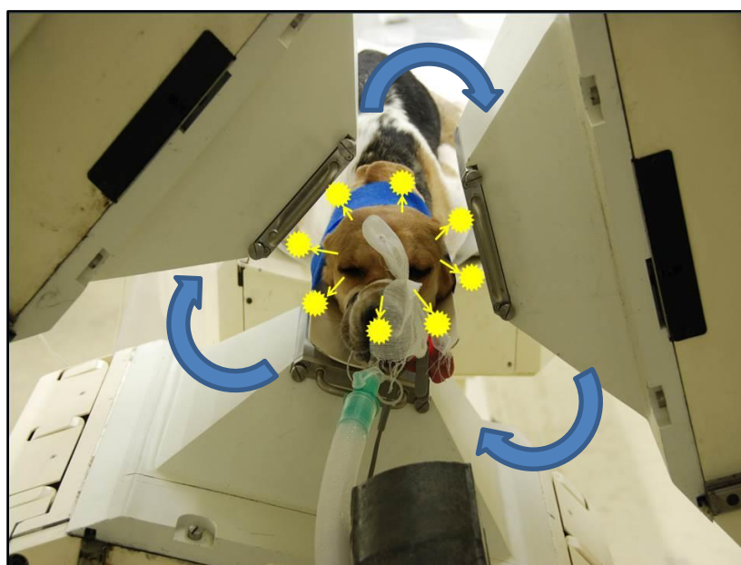
Figure 1: Photons emitted from the dog's brain (yellow dots) are registered by 3 detectors rotating around the head of the dog
