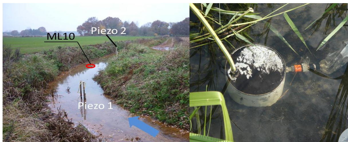
Figure 4.3: Streambed temperatures were measured at location ML10. Next to the temperature stick a seepage meter similar to the one shown here was installed into the streambed. Source: own .
