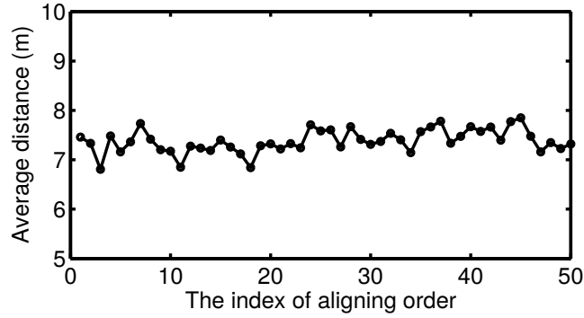
Figure 6.28: Influence of the aligning order using Method 1. No matter in which order the tracks are aligned, the average distance between all of the generated road segments and their ground truth is around 7.37 meters stably, which means the aligning order does not affect the track alignment significantly.
