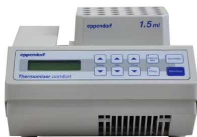
Figure 1.15. Eppendorf Thermomixer applied for the incubation of the in vitro metabolism studies.
