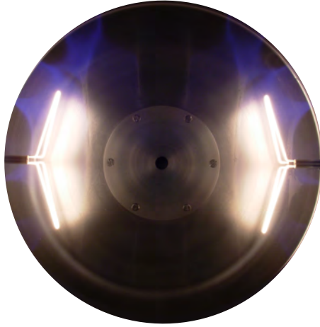
Figure 6.25: Photograph of the visible light emission pattern during an argon plasma in VISIONI reflecting the strong inhomogeneity of the ionizing electron density
