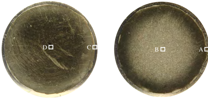
Figure 7.11: Photograph showing the two typical colour shade patterns found at the graphite sample surfaces after exposure to a deuterium plasma in VISIONI with impact energy per deuteron below (left) and above (right) the physical sputtering threshold for deuterium on carbon
