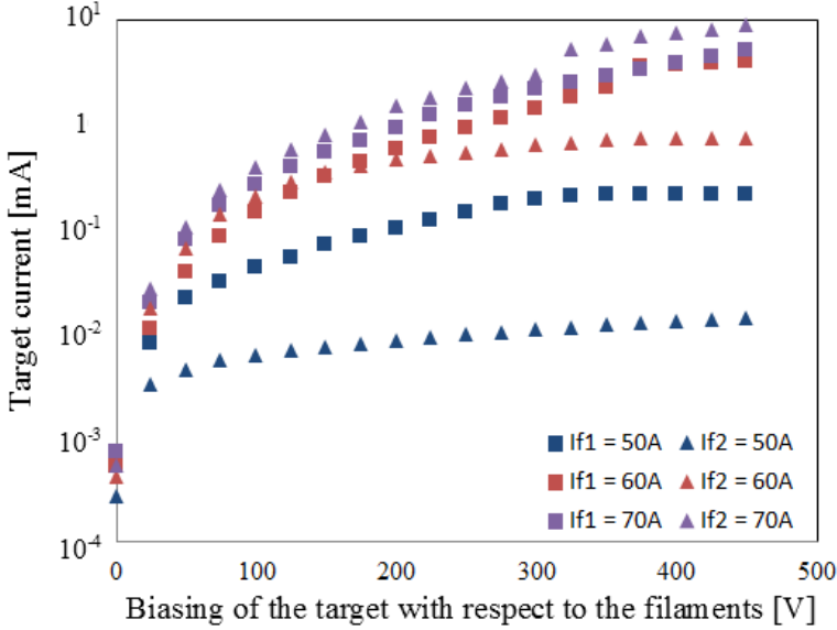
Figure 6.16: Target current measured in VISIONI as a function of the target biasing for different filament heating currents in order to determine the primary electron emission rate
