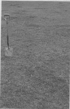
GOOD CONDITION VS = 2 Surface is relatively smooth and unbroken
