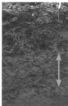
MODERATELY DEVELOPED HARD PAN The soil has a moderate penetration resistance to the knife. It is firm (hard) with a weakly apparent soil structure and has a soil porosity score of 0.5–1. There are few roots and old root channels, few worm channels, and few cracks and fissures. The pan may have few to common orange and grey mottles. Note the moderately developed tillage pan in the lower half of the topsoil (arrowed)
