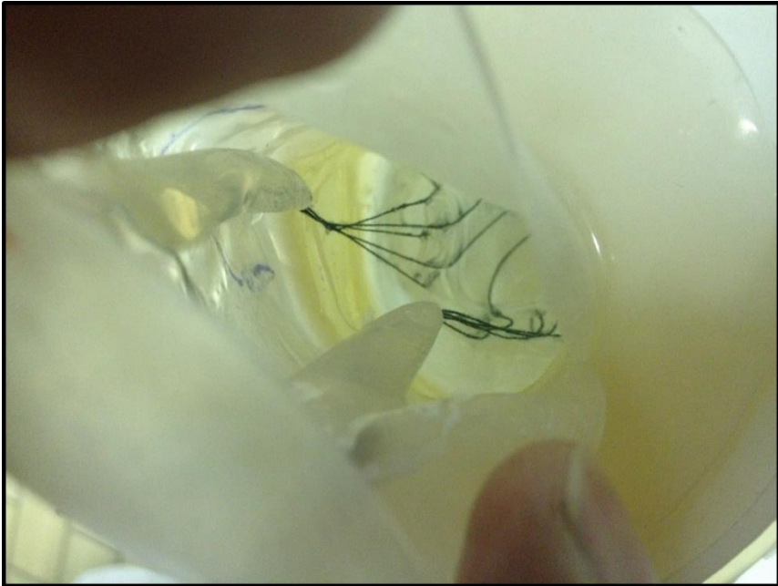
Figure 101: Attachment of the chordae tendineae of MV2 (Chapter 8) to the papillary muscles of the LH1 model.
