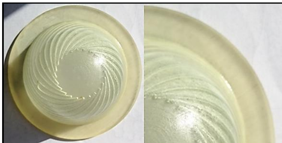
Figure 86: Design of the kernel according to the ViVitro left ventricular model geometry, which is used as a mold for the manufacturing of the actual model. The 24 fiber grooves at the inner side are clearly visible to enable accurate deposition of the fibers.
