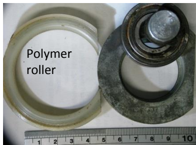
Figure A-2 dismantled roller assembly and part drawing of the polymer skeleton
