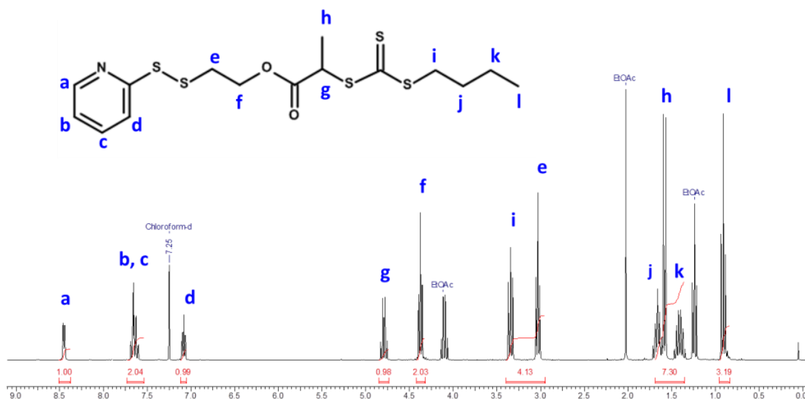
Figure 6. ^1\text{H-NMR} of PDS PABTC (300 MHz, \text{CDCl}_3 ) \delta (ppm): 8.46 (m, 1 H, H_{ortho-N} ), 7.70-7.60 (band, 2 H, H_{meta-N} and H_{para-N} ), 7.09 (ddd, J = 1.7, 4.9 and 6.6 Hz, 1 H, H_{ortho-disulfide} ), 4.80 (q, J = 7.4 Hz, 1 H, -\text{CHCH}_3 ), 4.38 (t, J = 6.4 Hz, 2 H, -\text{OCH}_2- ), 3.34 (t, J = 7.3 Hz, 2 H, -\text{SCH}_2\text{C}_3\text{H}_7 ), 3.03 (t, J = 6.4 Hz, 2 H, -\text{CH}_2\text{CH}_2\text{O}- ), 1.66 (app. quint, J = 7.3 Hz, 2 H, -\text{SCH}_2\text{CH}_2- ), 1.57 (d, J = 7.4 Hz, 3 H, -\text{CHCH}_3 ), 1.41 (app. sext, J = 7.3 Hz, -\text{CH}_2\text{CH}_3- ), 0.91 (t, J = 7.3 Hz, 3 H, -\text{CH}_2\text{CH}_3 ).
