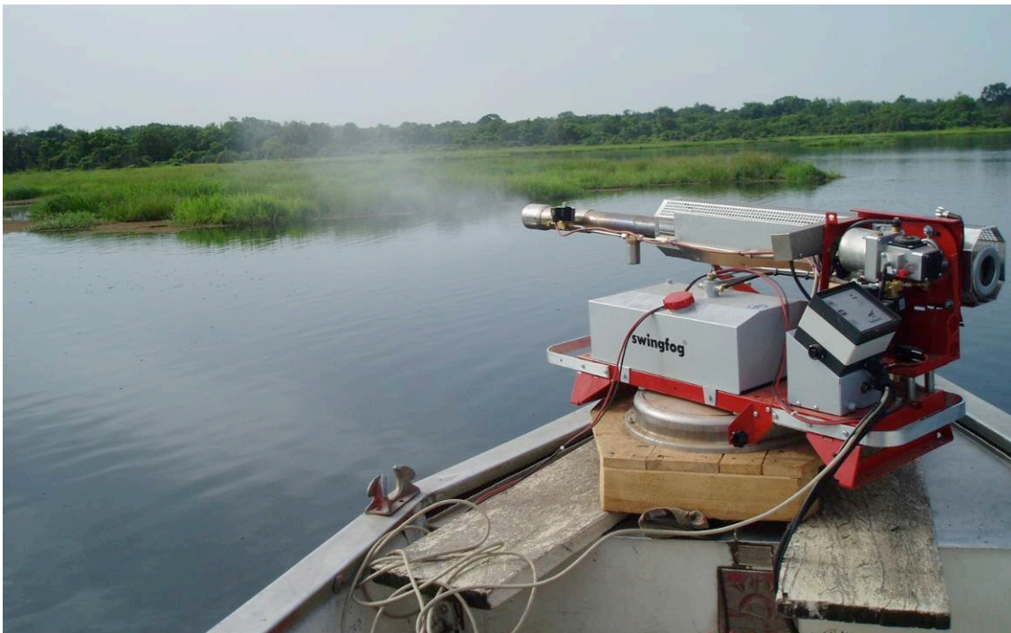
Figure 6. 3. Use of fogger (Swingfog ® ) in a boat on the Mouhoun River during PATTEC campaign
