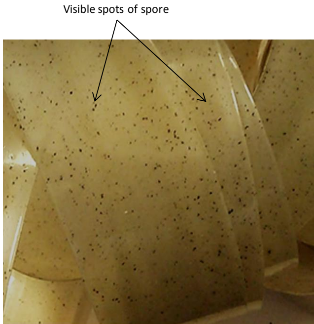
Figure 13. A photograph of PET film embedded with spores showing visible spots of spores on the film surface (indicated by arrows)
